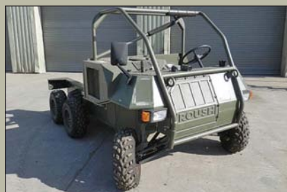
Roush 6x6 All terrain Load Carrier , Permanent 6 wheel Drive, Fully Automatic with Torque converter, Aluminium Honeycomb construction for lightweight and strength, McPherson Strut front Suspension, etc, Mileage From: 130km, Hours from: 60hrs, Year 2006, Excellent condition, Guide price from £12,500 (6 Available)
