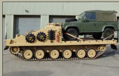
Alvis CVRT Shielder , Tracked Armoured load carrier with flat bed platform, The flat bed can adopted for a wide range of roles such as logistic carrier, bridge layer repair / recovery and towing. Built to a high specification the vehicle hull is composed of aluminium armour to protect the crew, etc. Mileage from 500, Excellent condition, Guide price from £15,000 (20 Available) .
